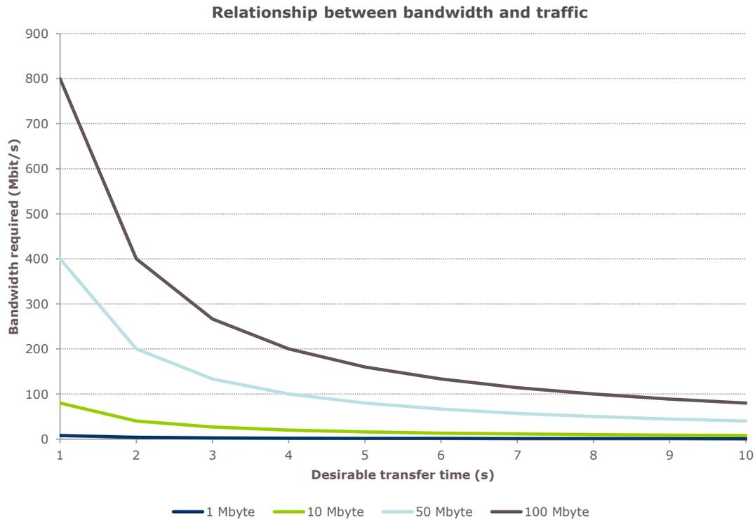
Figure 6. The relationship between bandwidth and traffic
