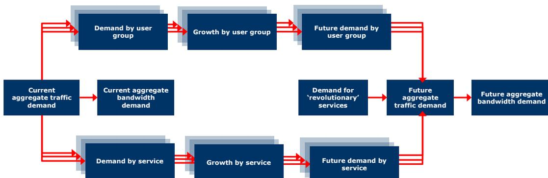
Figure 4. Schematic overview of the demand model
